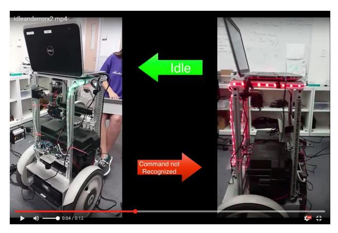
The idle command is shown to the left, using the wrap command and a 0 250 0 rgb value, shown when the robot is idle and waiting for a command. The wrong command is shown to the right, using the blink command and the 250 0 0 rgb value, shown when a command is not recognized.
