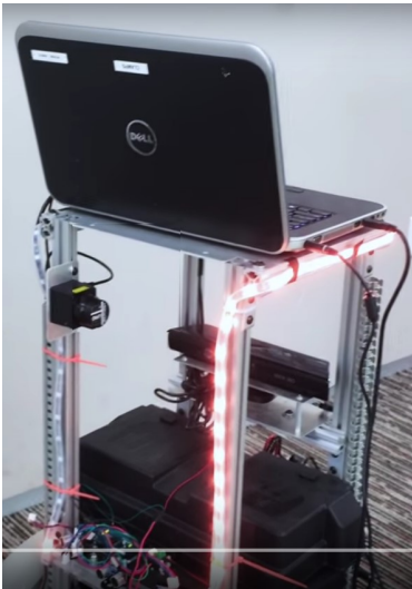
Figure 1: The placement of the LED light strip on the robot. The right turn signal is active in the figure.
