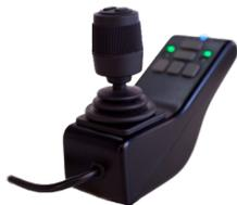
Figure 1: Built-in Kinova arm joystick.
