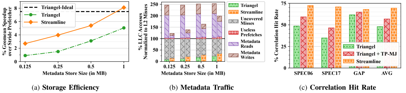
Fig. 13: Efficient Metadata Management: (a) Streamline matches Triangel's performance even when Streamline is given a metadata store that is half as large as Triangel's. (b) Streamline significantly reduces metadata traffic through its use of stream-based metadata and filtered indexing. (c) Streamline significantly improves correlation hit rate by considering prefetch utility in its replacement decisions.
