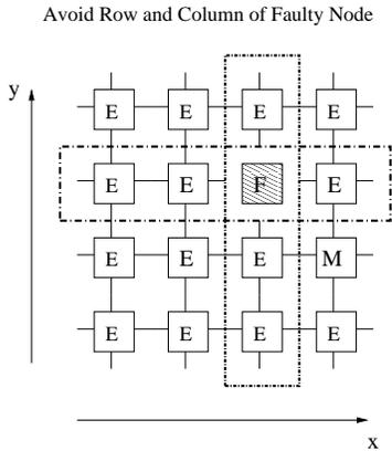
**Figure 5.** Avoid all the nodes in the same row or column as the faulty node during scheduling. This ensures that no communication path between a parent and child can include the defective node.
