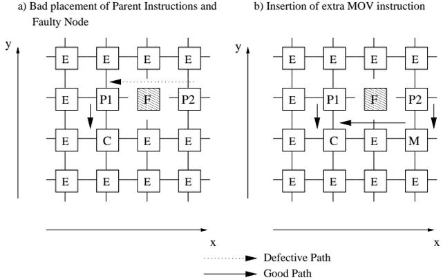
**Figure 4.** Figure 4a. shows that there is no path from the ALU corresponding to parent P2 to the child, since all paths have to pass through the faulty ALU. Figure 4b. shows the insertion of an extra *MOV* instruction that acts as an intermediate target. Both the routes from P2 to the *MOV* instruction and from the *MOV* instruction to the child are functional.
