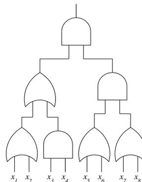
**Figure 1.** Tree representation of the formula  $((x_1 \vee x_2) \vee (x_3 \wedge x_4)) \wedge ((x_5 \vee x_6) \wedge (x_7 \vee x_8))$ . Only seven bits, representing the types of the gates, are needed to encode this formula.
