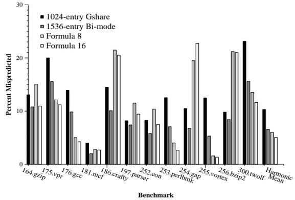
**Figure 6.** Accuracy of the predictors on each benchmark. This graph compares the Boolean formula predictor at history lengths of 8 and 16 against aggressively clocked implementations of *gshare* and bi-mode.
