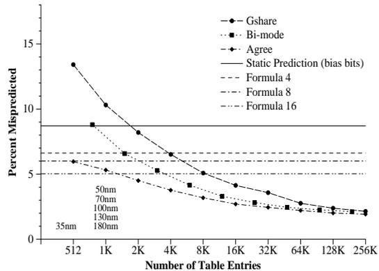
**Figure 4.** Accuracy of dynamic branch predictors vs. static prediction and the Boolean formula predictor. The numbers above the  $x$ -axis show the technologies in which the corresponding hardware budgets are reachable in one cycle with aggressive clocking. Misprediction rates are the harmonic means over the SPEC 2000 integer benchmarks.
