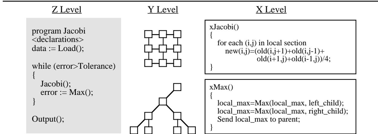
Figure 1: XYZ Illustration of the Jacobi Iteration
