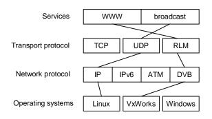
Figure 2 Interchangeable elements at each layer
