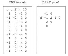
Fig. 1. DRAT-trim accepts two files as input: a formula in DIMACS CNF format (left), and a proof in the new DRAT format (right). Each line in the proof is either a lemma or a deletion step identified by the prefix "d". Spacing in both examples is to improve readability. If the RUP check fails, the DRAT-trim tool expects that a lemma has RAT on its first literal, as in the RAT format [2]. No check is performed for clause deletion steps, although the deleted clause needs to be present.
