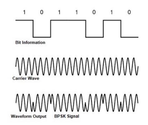
How to implement BPSK using Quadrature signal (ie, I & Q signal)?
