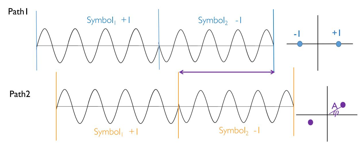
$-\sin(wt) + -\sin(wt + \theta) = A \sin(wt + \phi)$  causes change of amplitude A and shifted phase of  $\phi$
