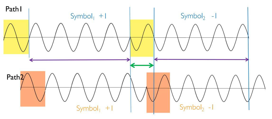
More than one cycles maybe repeated depending on the delay of path 2 signal
