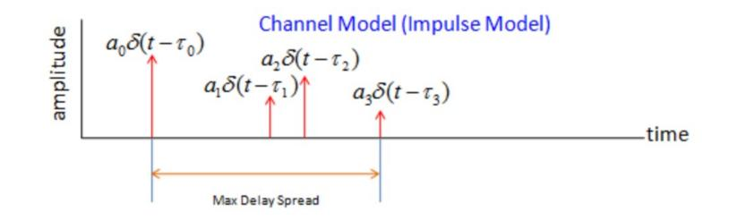
Cyclic prefix should span maximum delay spread
