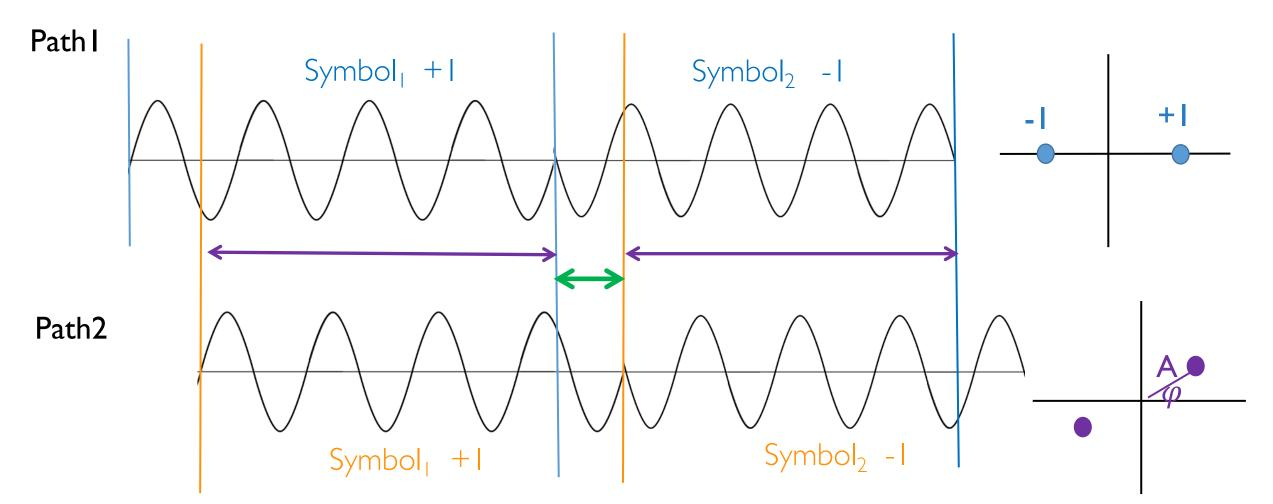
Both Path I signals and path 2 signal in PURPLE are continuous thus can be "equalized" However, they are DISCONTINUOUS in GREEN section which cannot be "equalized"
