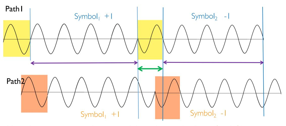
More than one cycles maybe repeated depending on the delay of path 2 signal
