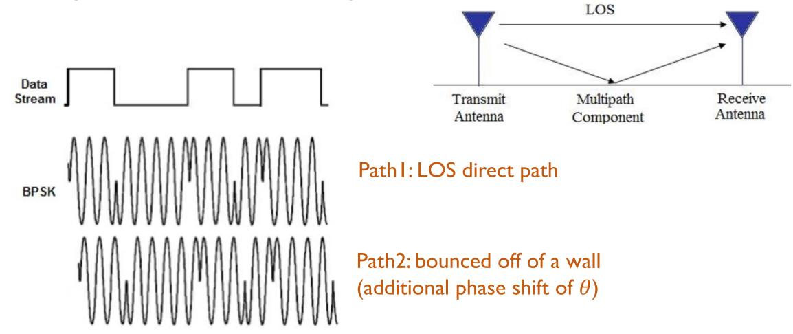
Signal from path I and signal from path2 are added together at the receiver
