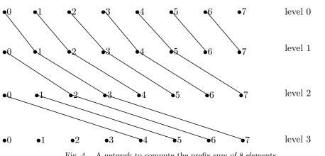
Fig. 4. A network to compute the prefix sum of 8 elements.
