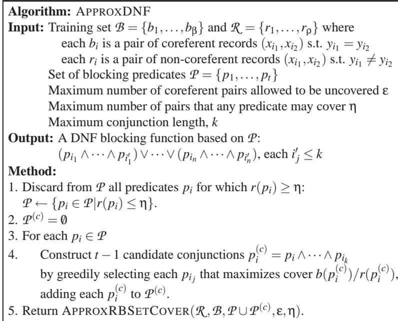
Figure 5.5: The algorithm for learning DNF blocking
