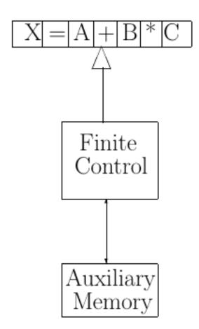
The *Finite Control* (a program with finite memory) reads symbols from the input tape one at a time, storing things in the *Auxiliary Memory*.
