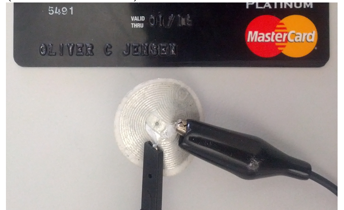
Figure 3: Eavesdropping Antenna (credit card for scale)
