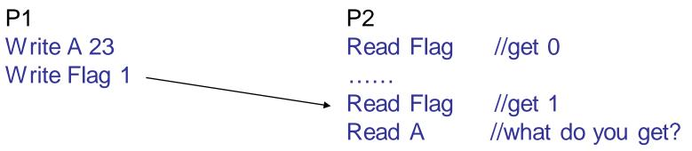
Problem: If the two writes on processor P1 can be reordered, it is possible for processor P2 to read 0 from variable A. Can happen on most modern processors.
