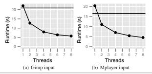
**Figure 15.** Points-to analysis times. Horizontal line is performance of the reference implementation. Best speedup over reference for gimp and mplayer are 3.63 and 3.62 respectively.
