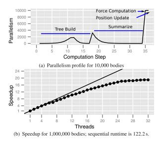
Figure 13. Parallelism profile and speedup for Barnes-Hut. All inputs initialized using the Plummer model.
