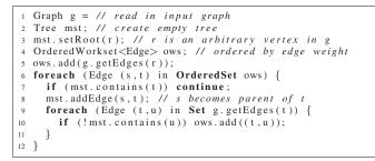
Figure 11. Top-down tree construction: Prim's MST algorithm
