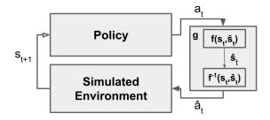
Figure : Modifiable simulator induced by GAT.
