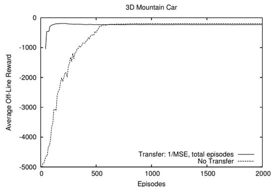
**Figure 5:** This graph compares learning without transfer to transfer using learned mappings. The transfer learning curve does not start at 0 episodes as it now reflects the total number of episodes used to learn the mappings in the source and target task. This result shows that the total time to learn a source task, an inter-task mapping, and then learn in a target task may less than learning a target task directly. Each learning curve averages 25 independent trials.
