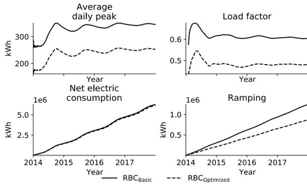
**Figure 4:** Energy flexibility performance metrics when the storage systems are controlled by the fixed log of either RBC<sub>Basic</sub> or RBC<sub>Optimized</sub> for the entire four year simulation period.
