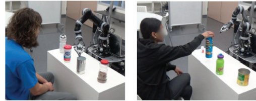
Fig. 12. (Left) The robot guesses an object described by a human participant as “silver, round, and empty.” (Right) A human participant guesses an object described by the robot as “light,” “tall,” and “tub.”
