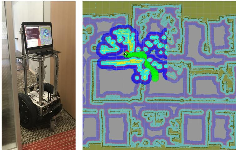
Figure 4: Left: Robot platform used in this research. Right: Occupancy-grid map (inflated) and a motion trajectory, indicated by a sequence of green planned for navigating through an office door.
