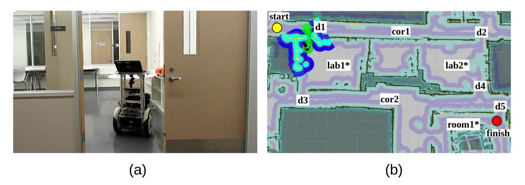
(a) A Segway-based robot preparing to go through a door
