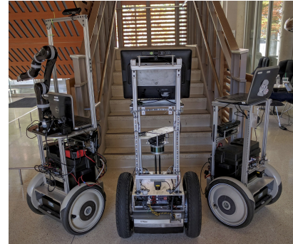
Fig. 1: The BWIBot family of robots. Left: V2 with Arm, Center: V3 (the robot used in this study), Right: V2.
