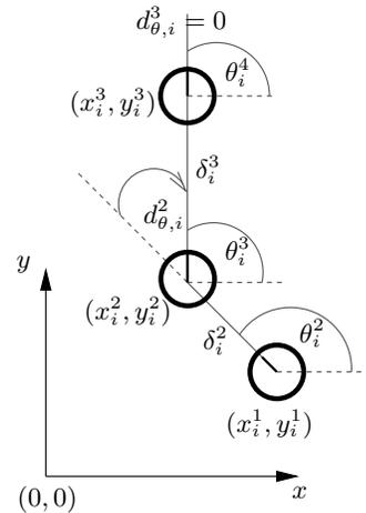
Fig. 1. Motion of robot  $i$  over a period of  $T = 3$  time steps, shown in a global coordinate system. The heading direction (bearing) is into the direction of the positive  $x$ -axis. For every time step  $t = 2, \dots, T$ , the robot can observe the relative change in direction  $d_{\theta,i}^t = d_{\theta}(i, t)$ , and the amount of distance traveled  $\delta_i^t = \delta(i, t)$ . In general, the initial pose  $(x_i^1, y_i^1, \theta_i^2)$  will be unobservable.
