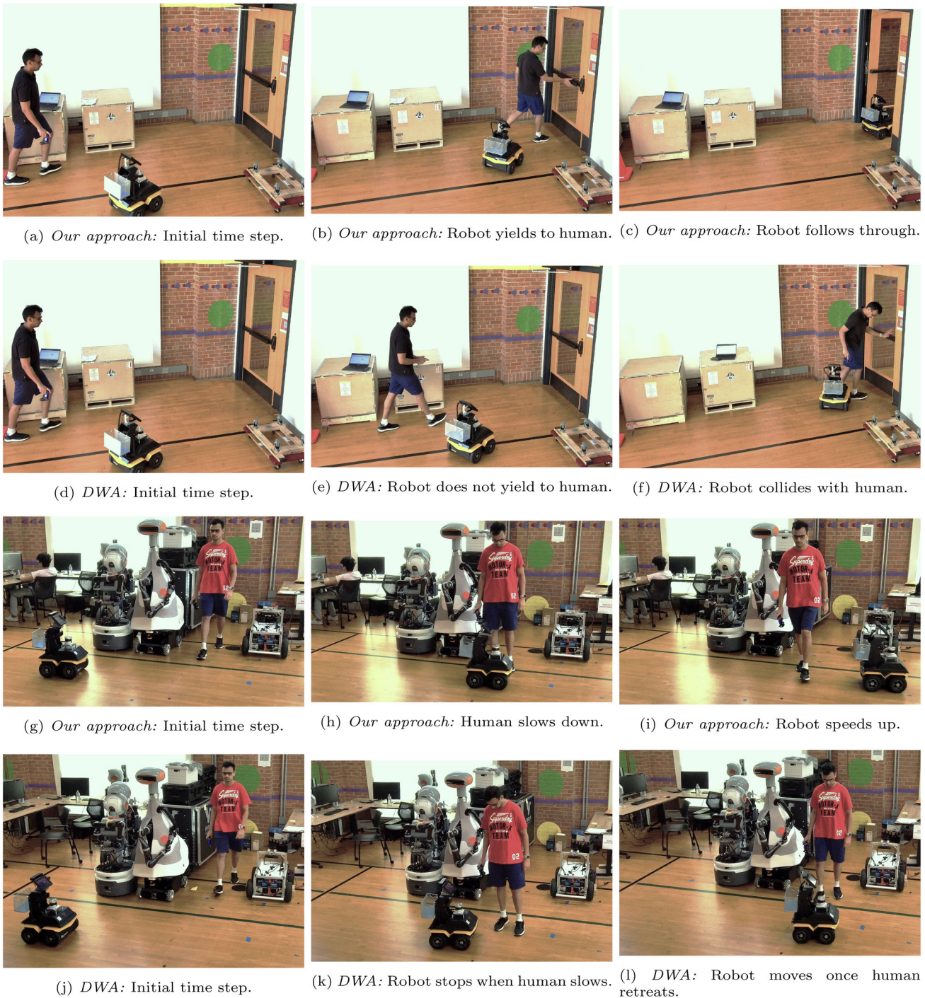
Fig. 10 Deployment in human-robot scenarios: ( Doorway ) Figs. 10a, 10b, and 10c demonstrate our deadlock avoiding strategy enables the robot to yield to the human by slowing down, rather than stopping, and smoothly follows the human through the door. Figures 10d, 10e, and 10f demonstrates a baseline DWA planner that results in the robot stopping abruptly in front of the human, only moving forward once the human steps back. ( Intersection ) Figs. 10j, 10k, and 10l demonstrate our
