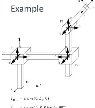
$$\begin{split} T_{0,1} &= trans(0, L_1, 0) \\ T_{1,2} &= trans(l_2, 0, 0)rot(z, 90^\circ) \\ T_{2,3} &= trans(l_3, 0, 0)rot(z, -90^\circ + \theta_1) \\ T_{3,T} &= trans(L_4, 0, 0)rot(z, 90^\circ)rot(x, 90^\circ) \end{split}$$
