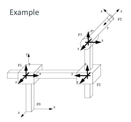
$$\begin{split} T_{0,\,1} &= trans(0,L_1,0) \\ T_{1,\,2} &= trans(l_2,0,0)rot(z,90^\circ) \\ T_{2,\,3} &= trans(l_3,0,0)rot(z,-90^\circ+\theta_1) \\ T_{3,\,T} &= trans(L_4,0,0)rot(z,90^\circ)rot(x,90^\circ) \end{split}$$
