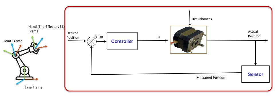
Tasks are usually defined in 3D Cartesian Space not joint space We want to move a frame on the robot to a desired pose We need to deal with poses and motion in Cartesian space
