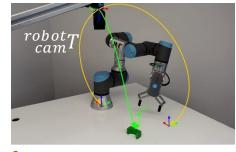
$$^{robot}p = {^{robot}_{cam}}T^{cam}p$$
