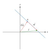
• To define a motion, we need to define the line and the amount of motion. Start by defining that line in standard parametric form
