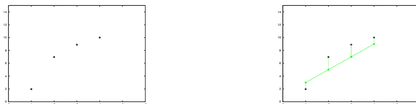
Figure 6.2: Left: A plot of the points. Right: Some first guess of a line that interpolates, and the distance from the points to the line.
