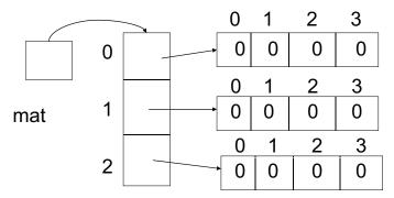
$\tt mat$  holds the memory address of an array with 3 elements. Each element holds the memory address of an array of 4 <code>ints</code>
