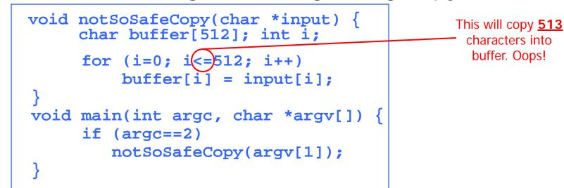
1-byte overflow: can't change RET, but can change pointer to <u>previous</u> stack frame
