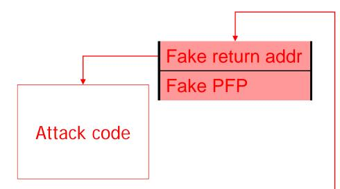
Change the caller's saved frame pointer to point to attack-controlled memory. Caller's return address will be read from this memory.
