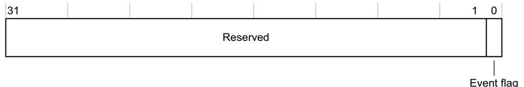
**Figure 4-4 Watchdog Interrupt Status Register bit assignment**
