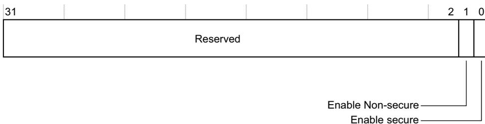
**Figure 3-1 ICDDCR bit assignments for Secure accesses**
