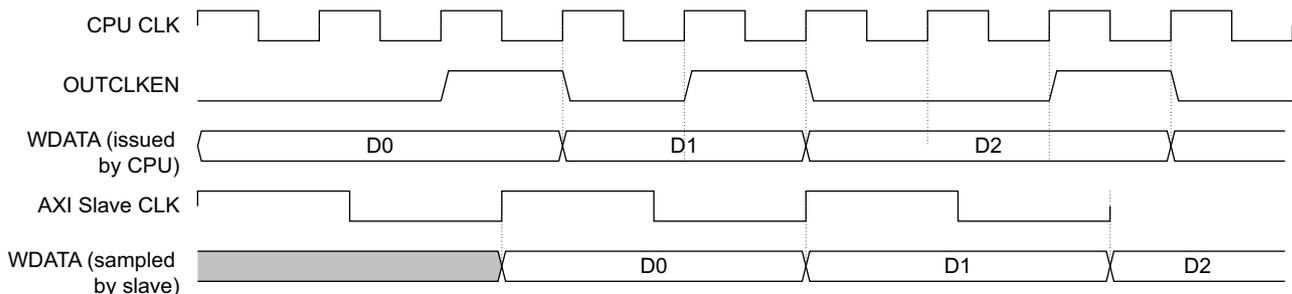
Figure 2-12 Timing diagram for OUTCLKEN with five-to-two clock ratio between CPU and AXI Slave CLK
