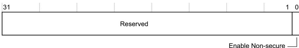
**Figure 3-2 ICDDCR bit assignments for Non-secure accesses**
