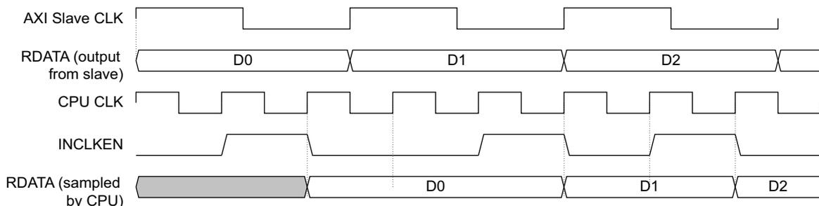
**Figure 2-10** Timing diagram for INCLKEN with five-to-two clock ratio between CPU and AXI Slave CLK
