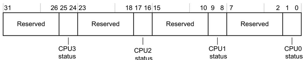
Figure 2-3 SCU CPU Power Status Register bit assignments
