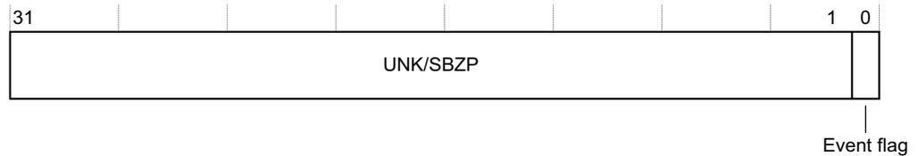
**Figure 4-2 Private Timer Interrupt Status Register bit assignment**
