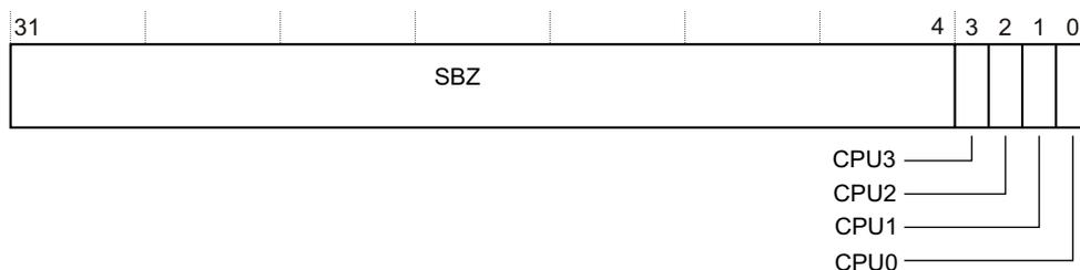
Figure 2-7 SAC register bit assignments
