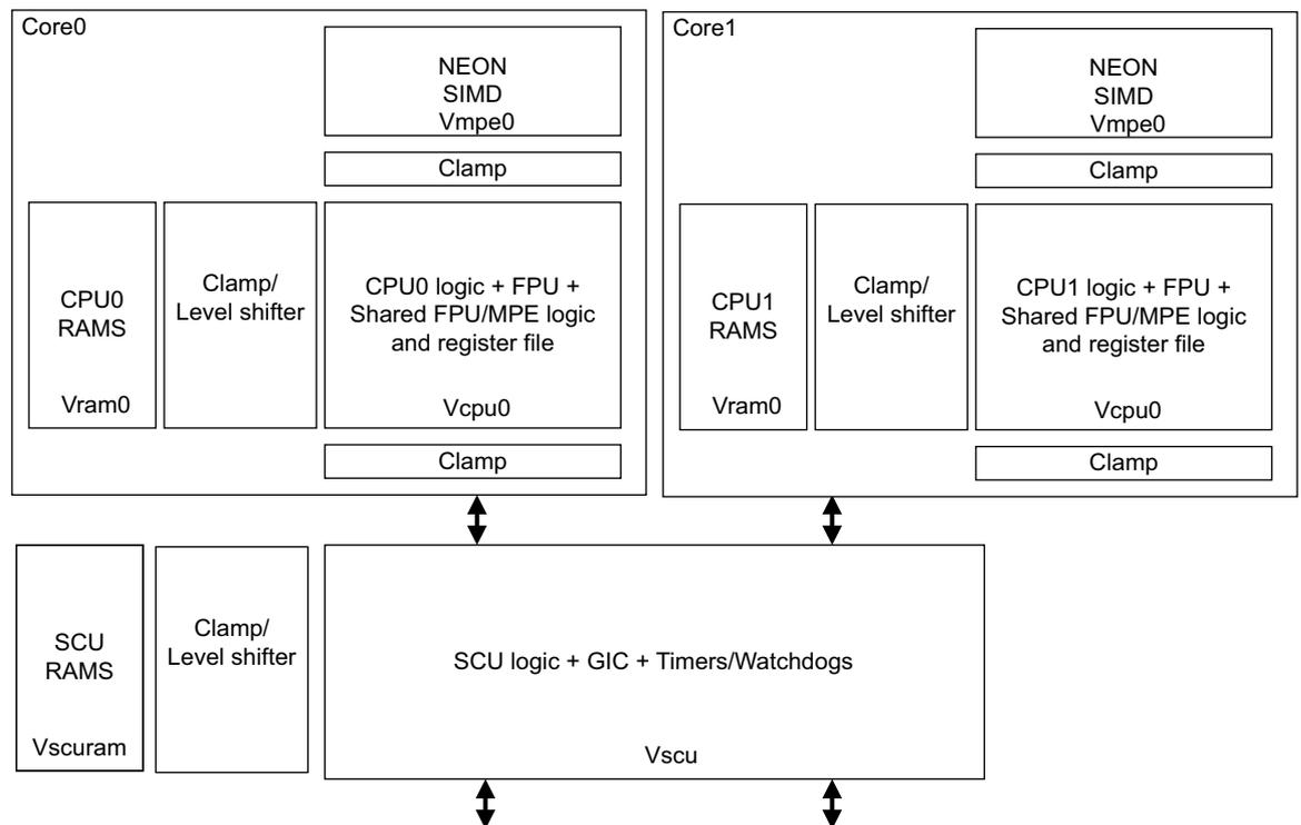
Figure 5-2 Cortex-A9 MPCore power domains and clamps
