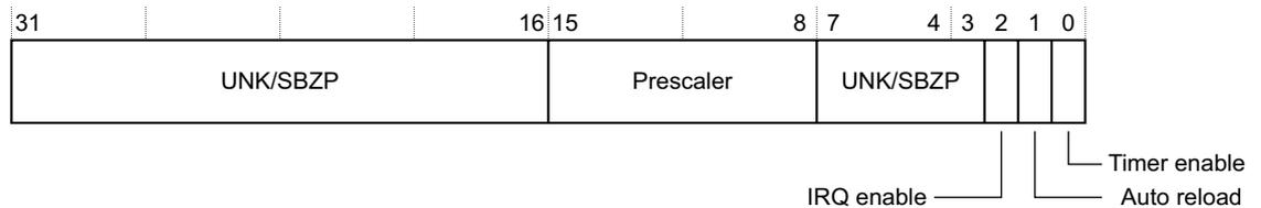
Figure 4-1 Private Timer Control Register bit assignments
