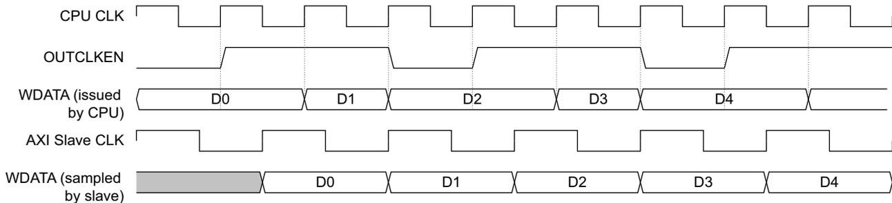
Figure 2-11 Timing diagram for OUTCLKEN with three-to-two clock ratio between CPU and AXI Slave CLK
