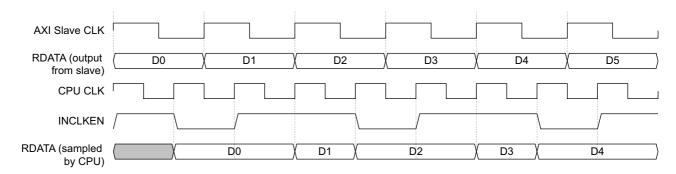
Figure 2-9 Timing diagram for INCLKEN with three-to-two clock ratio between CPU and AXI Slave CLK
