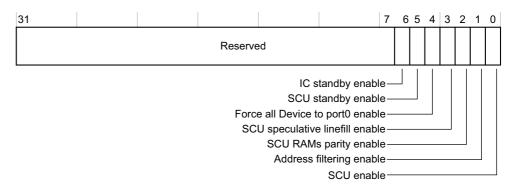
Figure 2-1 SCU Control Register bit assignments
