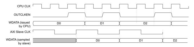
Figure 2-12 Timing diagram for OUTCLKEN with five-to-two clock ratio between CPU and AXI Slave CLK
