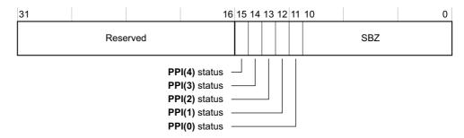
Figure 3-5 ICPPISR bit assignments
