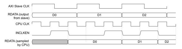
Figure 2-10 Timing diagram for INCLKEN with five-to-two clock ratio between CPU and AXI Slave CLK
