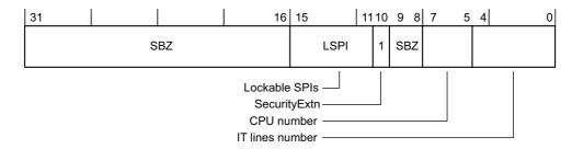
Figure 3-3 ICDICTR bit assignments
