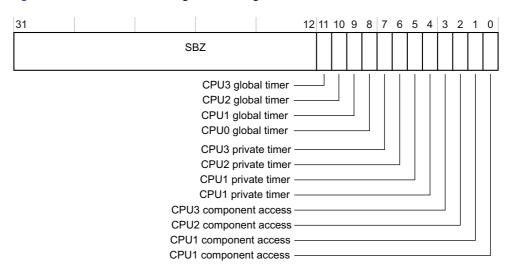
Figure 2-8 SNSAC register bit assignments
