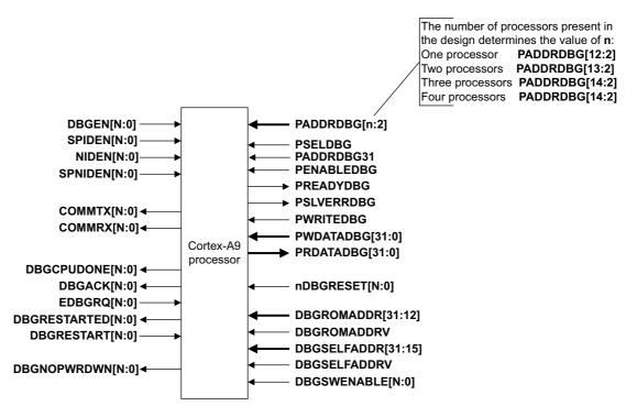
Figure 6-1 External debug interface signals in CortexA9 MPCore designs
