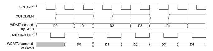
Figure 2-11 Timing diagram for OUTCLKEN with three-to-two clock ratio between CPU and AXI Slave CLK
