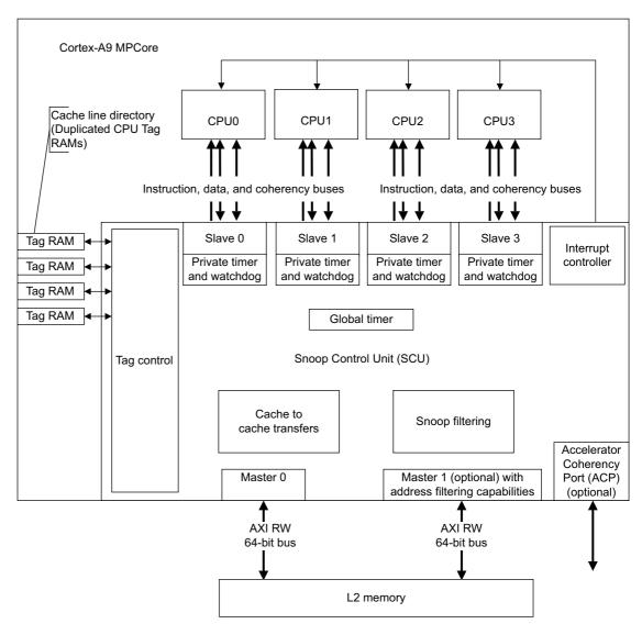
Figure 1-1 Example multiprocessor configuration
