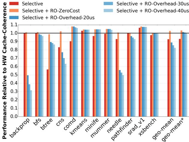
Figure 8: GPU performance when using Selective caching (Request-Coalescing + 512kB-CC + Variable-Transfers) combined with read-only caching. `geo-mean*`: Geometric mean excluding `backprop`, `cns`, `needle`, where read-only caching should be disabled. (RO: Read-Only)
