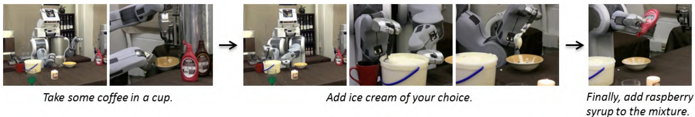
Fig. 4. Robot Experiment. Given the language instruction for making the dessert ‘Affogato’: ‘ Take some coffee in a cup. Add icecream of your choice. Finally, add raspberry syrup to the mixture. ’, our algorithm outputs a sequence that the PR2 executes to make the dessert. (Please see the video.)
