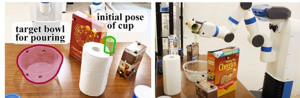
Fig. 1. A pouring demonstration in a cluttered tabletop environment. The robot has to execute a motion that *pours* the contents of the cup into the bowl, while avoiding the clutter in the scene.
