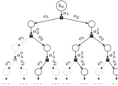
Fig. 2: A full conditional plan  $\gamma_k$  contains both solid and dotted branches.  $a_1, a_2^0, \dots$  are actions.  $o_1$  and  $o_2$  are observations. A partial conditional plan  $\gamma_k^p$  contains only solid branches.
