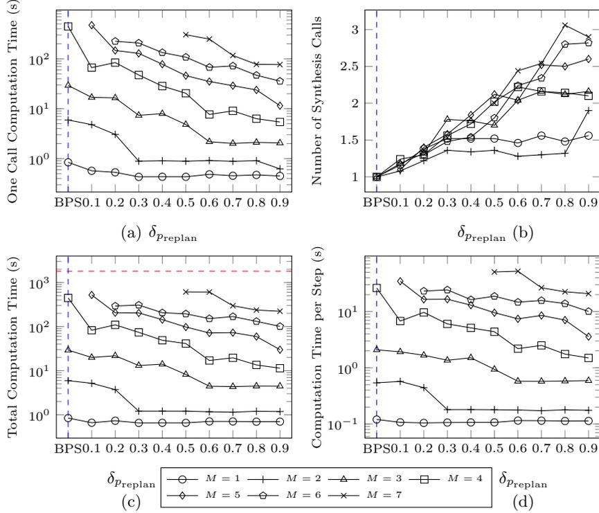
Fig. 5: Performance results for the kitchen domain as the bound  $\delta_{p_{\text{replan}}}$  increases. Different plots correspond to tests with different numbers  $M$  of obstacles. Missing data points in a plot indicate time-out. The red dashed line is the plot of time = 1800 seconds (time-out). The blue dashed line passes through the data points generated by BPS. All the results are averaged over 50 independent runs.
