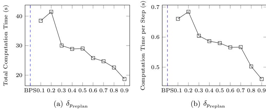
Fig. 9: Performance results for the Tag domain as the replanning probability bound  $\delta_{p_{\text{replan}}}$  increases. All the results are averaged over 50 independent runs.
