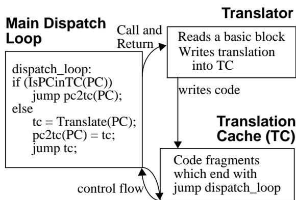
**FIGURE 3.2. Main loop of a dynamic translation simulator**
