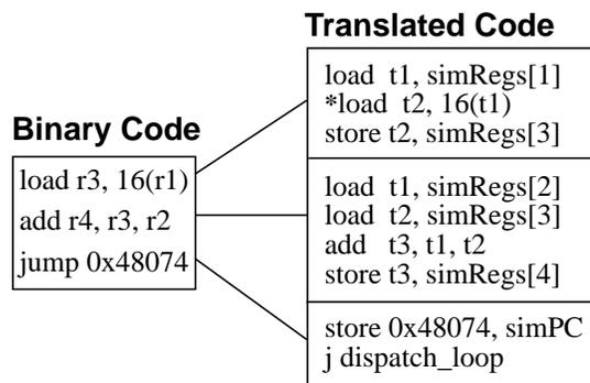
**FIGURE 3.1. Instruction set simulation using binary translation**
