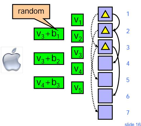
Blinded attribute values are converted to Yao circuit inputs using oblivious transfer
