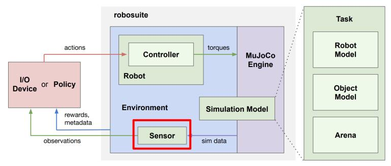
Retrieve information generate observations as the physical signals such as RGB-D cameras, force-torque measurements, and proprioceptive data.
