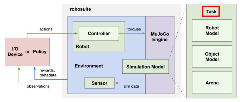
encapsulates three essential constituents of robotic simulation: Robot Models(1+), Object Models(0+), and Arena(1).
