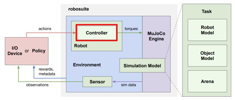
Interpret the action commands and transform them into the low-level torques passing to the underlying physics engine
