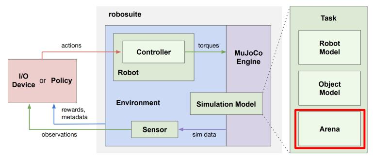
defines the workspace of the robot, including the environment fixtures, such as a tabletop, and their placements
