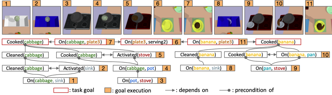
Figure 4: Visualization of RPN solving a sample cooking task with one dish and two ingredients ( I = 2 , D = 1 ): (Top) Visualization of the environment after a goal is achieved (zoom in to see details), and (Bottom) the regression planning trace generated by RPN. Additional video illustration is in the supplementary material.
