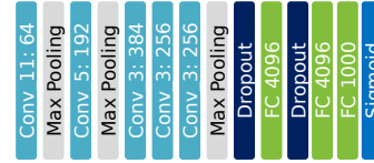
Figure 3: The architecture of our deep attribute CNN model.
